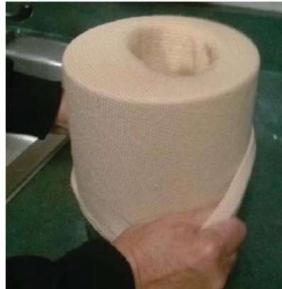
3. Pull the edges of the shrinker sock all the way down the sides of the tube until the end of it is flat on top.
