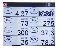
**S<sub>VD</sub>O<sub>2</sub> (%)** oxygen saturation of blood in the venous drainage tubing
